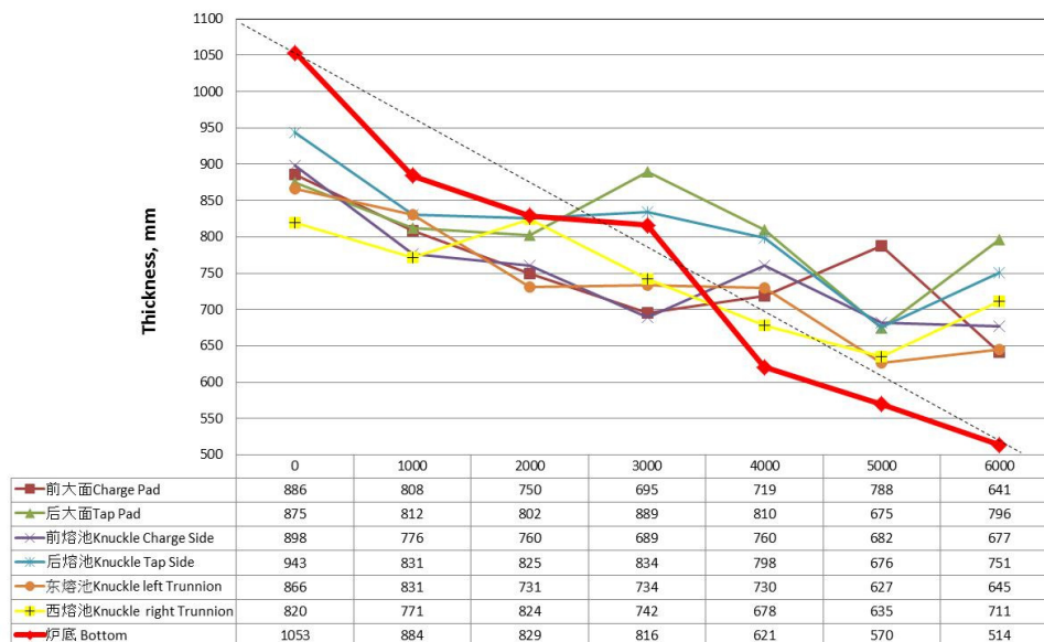
Figure 11: Wear profile development in the recent campaign of #3BOF at Meishan steel
