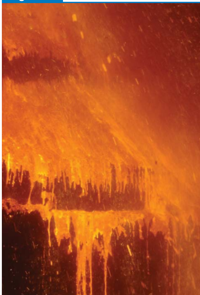
Heavy slopping caused by high slag volume.
