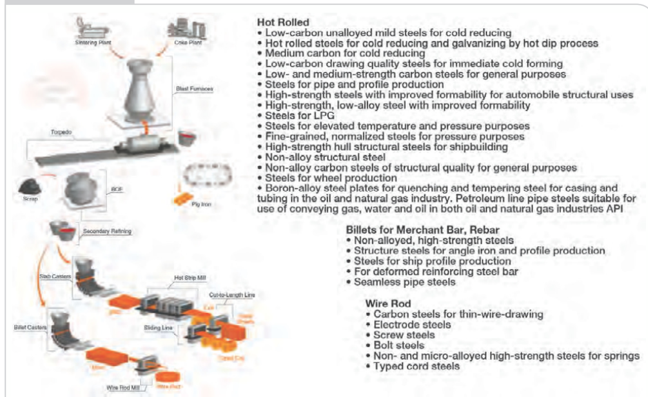
Process flow and metallurgical facilities at Isdemir.
